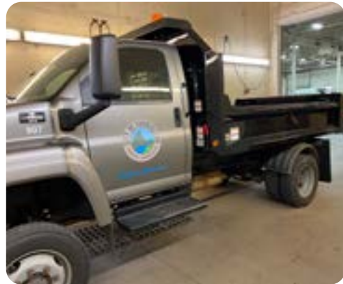
Henderson dump body replaced rusted dump body on 2007 truck with only 55,000 miles.
